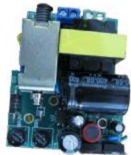
Remote reset circuit PT500-20
